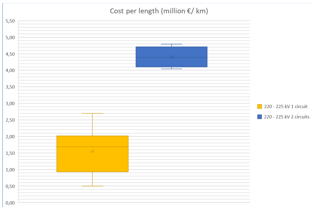
Figure 6. UIC indicators for underground cables of 220-225 kV voltage range with 1 and 2 installed circuits; million EUR/km
