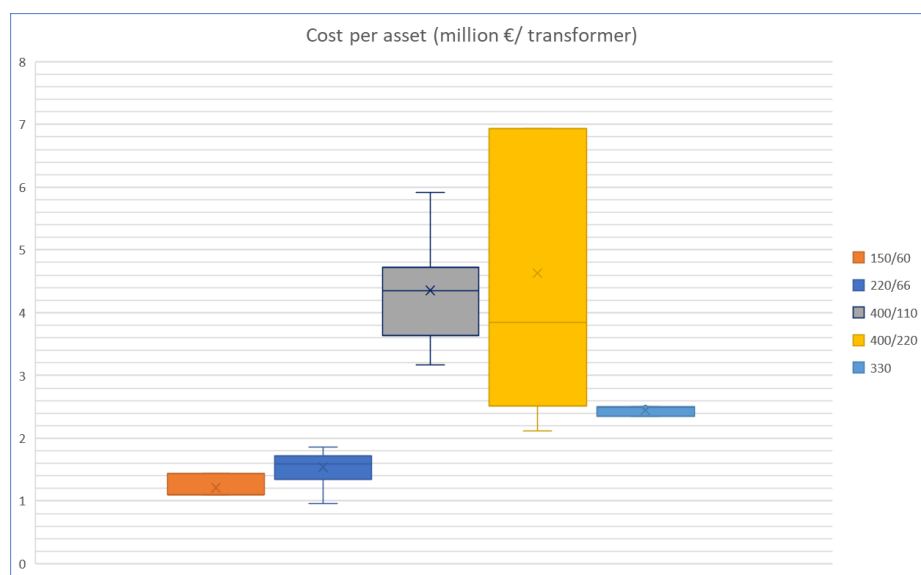
Figure 13. Comparison of UIC for transformers per voltage level; million EUR/transformer
