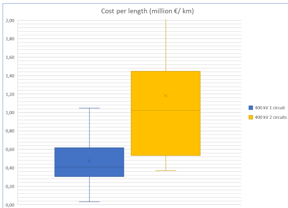
Figure 3. UIC indicators for overhead lines of 380 - 400 kV with 1 and 2 installed circuits; million EUR/km
