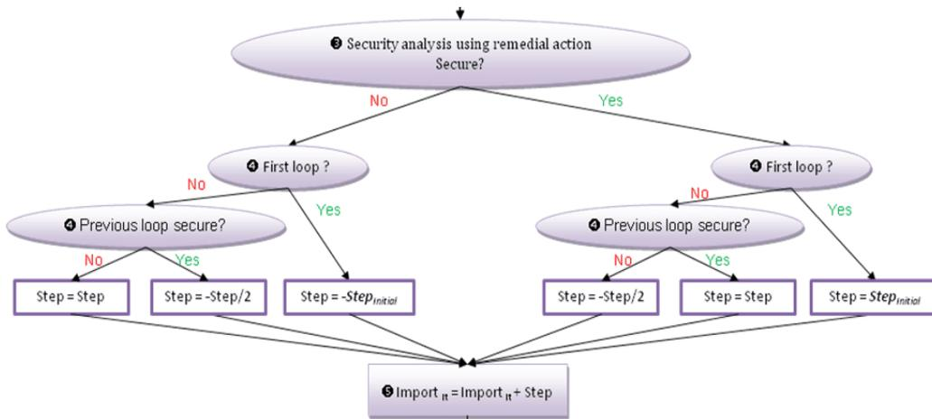
The dichotomy is set with a 50 MW step in order to optimize the capacity offered to the market while reducing the computation time. Considering optimal remedial actions have been applied in each step of CC, the dichotomy approach guaranties final solution is less than 50 MW suboptimal compared to absolute maximum Italian import.
