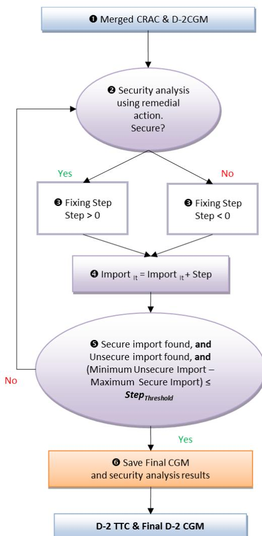
If the level is secure or can be made secure by optimizing remedial actions, the coordinated capacity calculator will then test a higher value of TTC. Otherwise, it will then test a TTC value in between the
