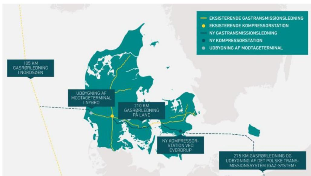
Figure 2 Representation of the Danish transmission network showing point locations and distances.
