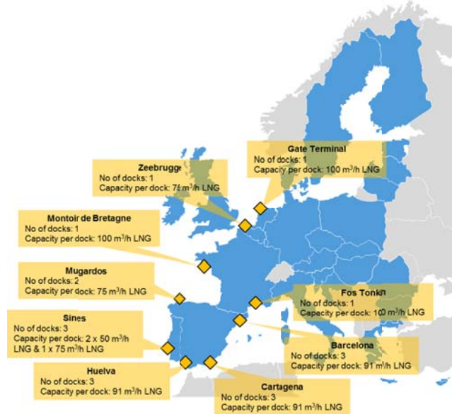
Figure 9: EU LNG Terminals with truck loading facilities (Source: GIE)
