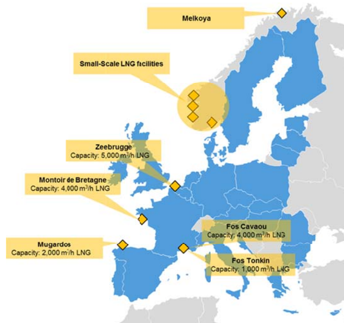
Figure 27: LNG bunkering facilities in the EU and Norway (Source: Gas Infrastructure Europe, Gasnor)
