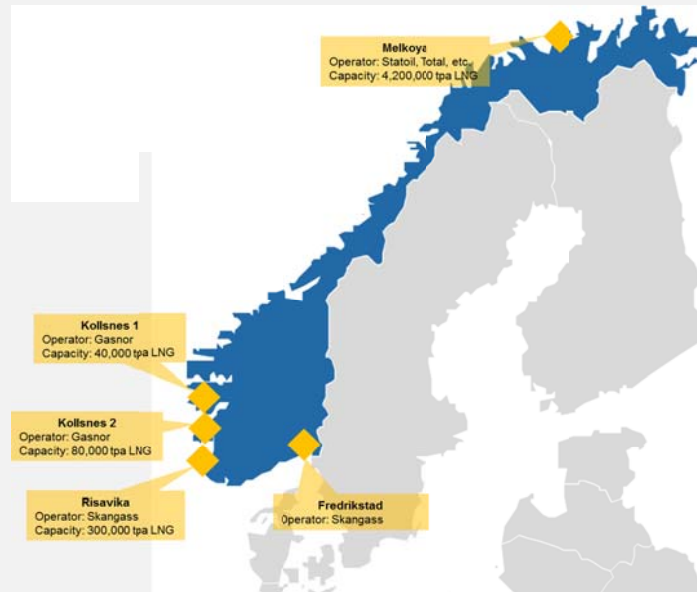
Figure 29: Liquefaction plants in Norway (Source: Gasnor)
