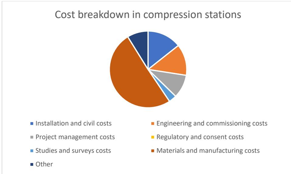
Figure 26. Cost breakdown in compression stations (<1MW); in%
