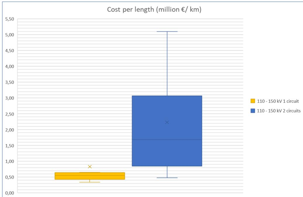
Figure 5. UIC indicators for underground cables of 110-150 kV voltage range with 1 and 2 installed circuits; million EUR/km
