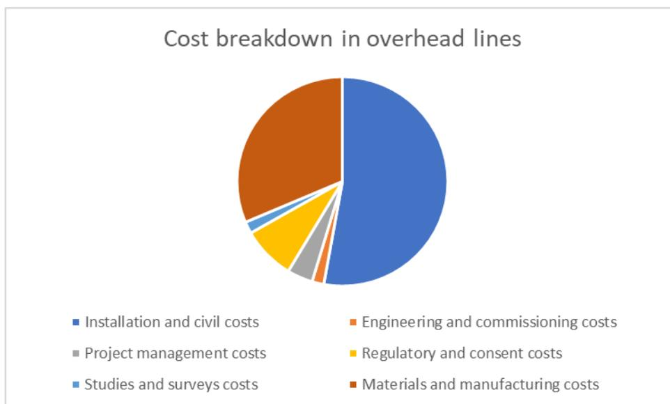
Figure 20. Cost breakdown in overhead lines; in %
