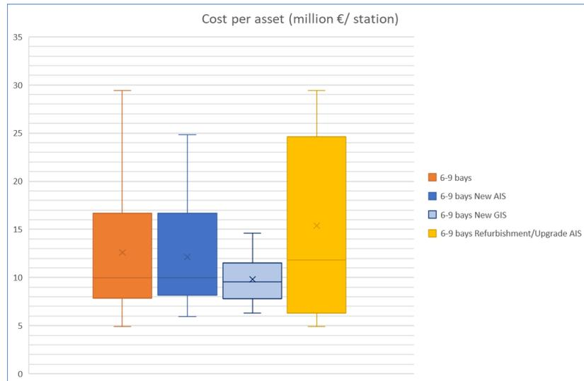
Figure 11. UIC indicators for AC substations with 6-9 bays per type, new and upgraded/refurbished; million EUR/station
