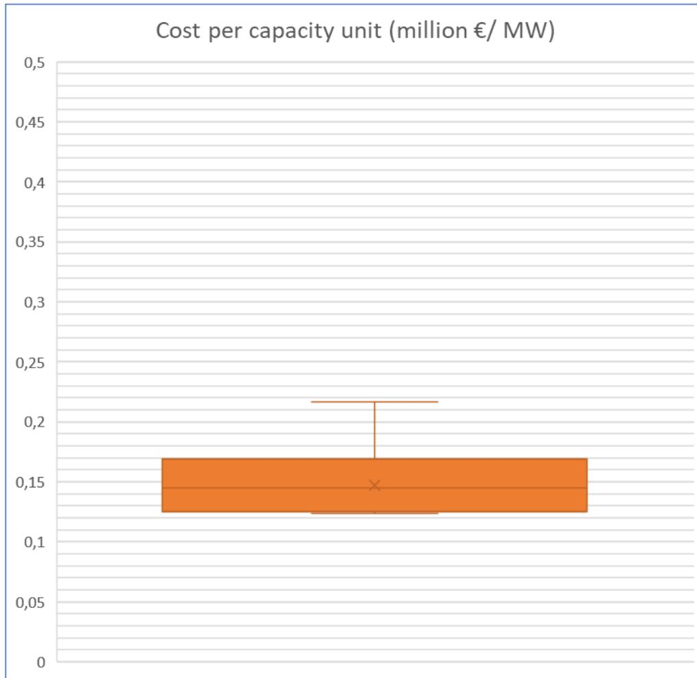
Figure 15. UIC indicators for HVDC converters; million EUR/ MW
