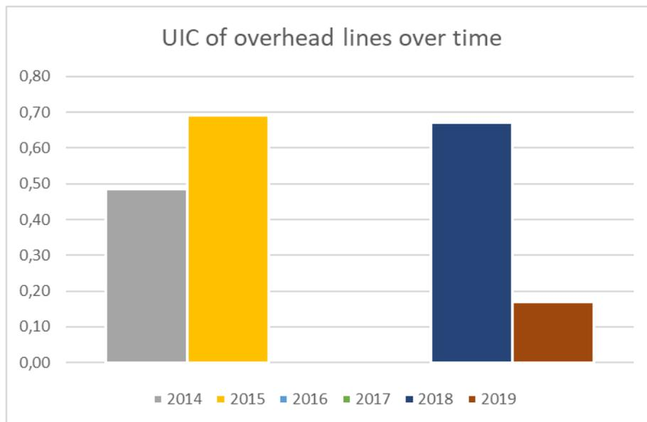
Figure 21. Average UIC of overhead lines (220 kV and 2 circuits) per annum; in million EUR/km
