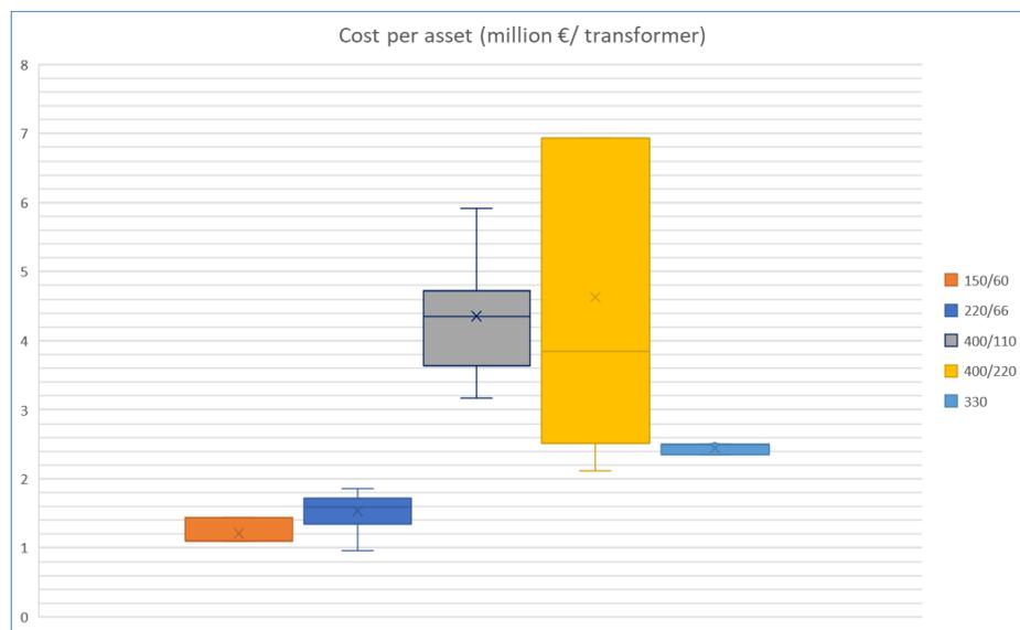
Figure 13. Comparison of UIC for transformers per voltage level; million EUR/transformer
