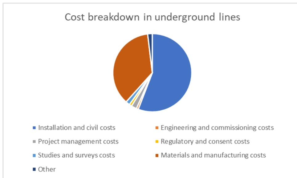
Figure 23. Cost breakdown in underground cables; in %
