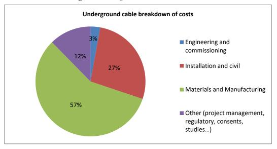
Figure 4: Underground cable cost breakdown
