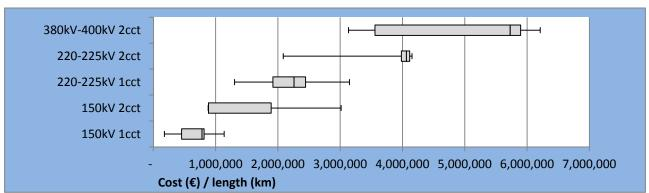
$Figure \ 3: \ Underground \ cables \ by \ route \ length \ (km) \ by \ quartile \ box-plots$
