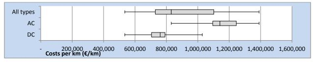
Figure 6: Subsea cable cost breakdown
