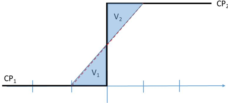
If we assume a predefined ramping period,  $RP$ , symmetrical around the ISP shift, the ramping energy volume faced by a TSO,  $V_{ramp}$ , can be defined as the sum of volume  $V_1$  and  $V_2$  in the figure, where the two volumes are equal.
