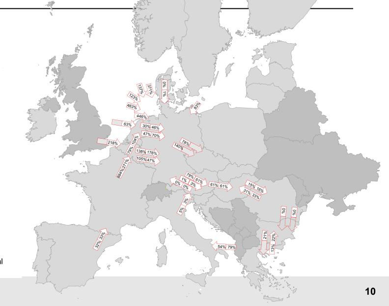
Utilisation rate (%) is average physical flow / maximum firm technical Source: ENTSOG TP
