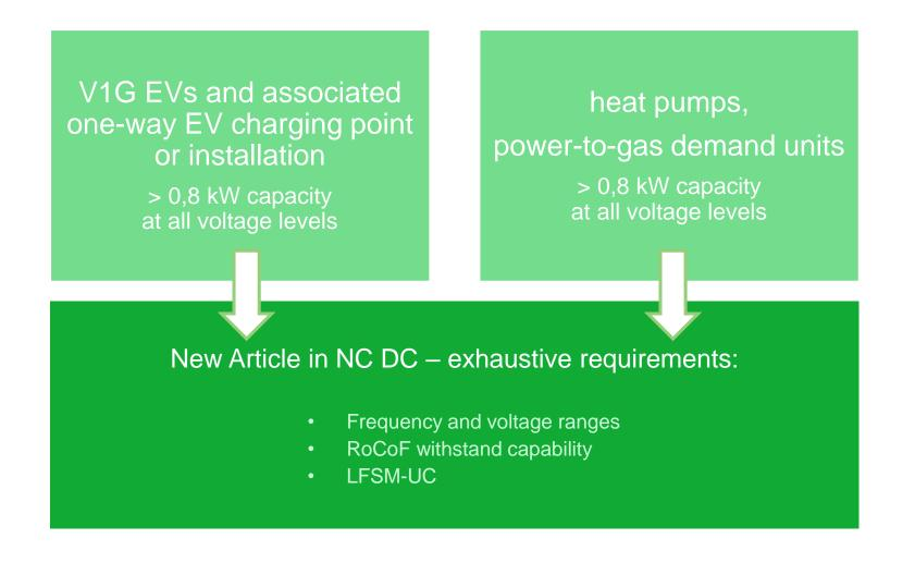
**0,8 kW** – capacity threshold follows the current NC RfG determination of significance rules
