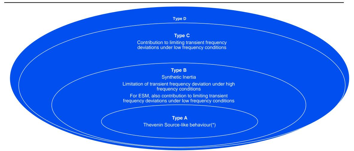
(\*) the instantaneous AC voltage characteristics of the internal Thevenin source shall be capable of not changing its amplitude and voltage phase angle while voltage phase angle steps or voltage magnitude steps are occurring at the connection point.
